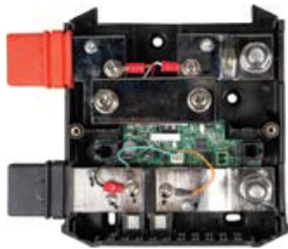
Lynx Shunt VE.Can (M10) with fuse dummy busbar installed
